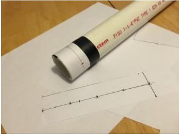
Next you will do almost the same again, this time you will cut a 50mm wide strip of paper. Make two parallel lines on the paper exactly 24mm apart. Take your measurement (Circumference divided by 4) and mark your drill points on the paper, this time staggering the points between the two lines.
