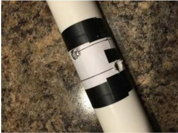
Lastly, you will need to drill holes for the coax balun. This can be done anywhere on the pipe, but I did it about 6 inches below the top holes. Take your coax and wrap it around the pipe so the end result will be 4 complete turns and mark where the coax will go through. After this step you might want to consider painting the PVC pipe. I will generally use a fine sandpaper then spray paint it with
