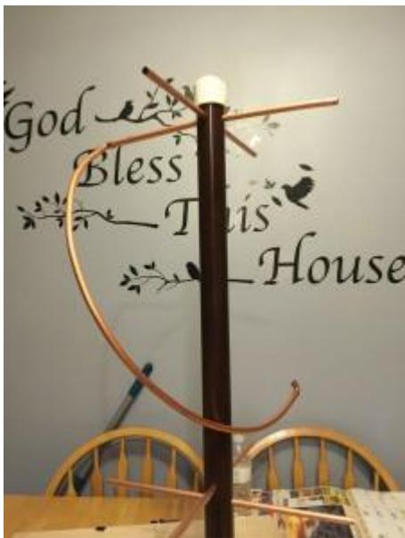
Grasp the top connection with one hand and gently bend the 812mm piece to meet the lower cross bar on the opposite side. You must bend the ENTIRE antenna ANTI-CLOCKWISE when viewed from the top. I repeat, you must bend each leg ANTI-CLOCKWISE. The bend should be as even as possible, and I frankly don't have any magic way to get this done or confirm it was done correctly other than the old hairy eyeball.
